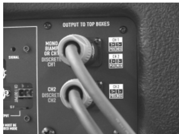
Speakons provide a clean appearance, reliable electrical connection and positive locking mechanism. To remove a Speakon, pull the thumb-latch back and twist counterclockwise 1/8th turn.
